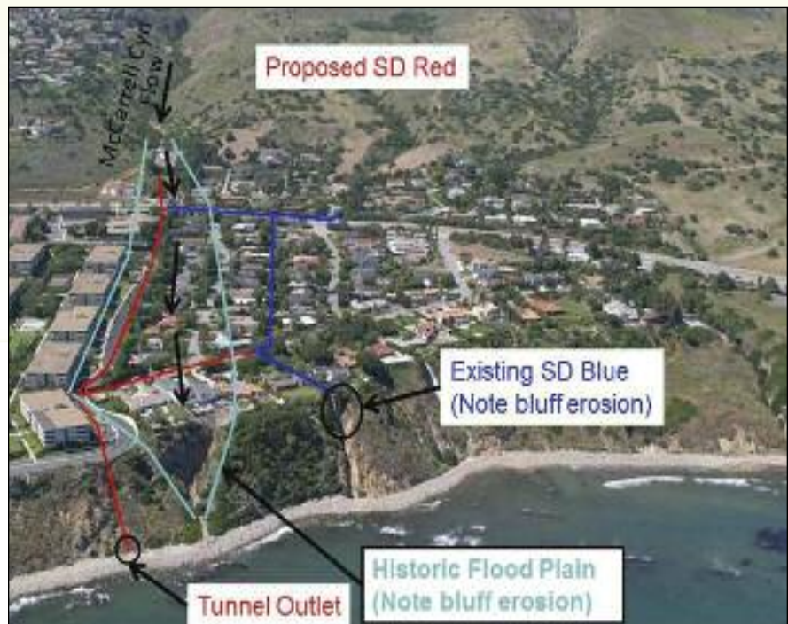
McCarrell Canyon Storm Drain System with Historical Flood Plain in Light Blue
